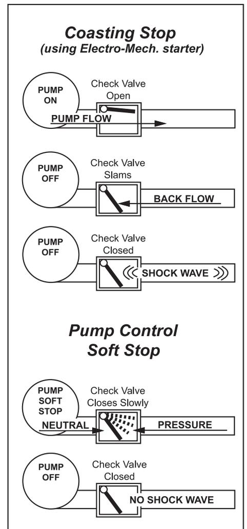
By using the Soft Stop/Deceleration feature of the **ASAMV**, the pump output torque is gradually and gently reduced, which slowly reduces the pressure in the pipe. When the Output Pressure is just slightly lower than the Head Pressure, the flow slowly reverses and closes the Check Valve. By this time there is very little energy left in the moving fluid and the Shock Wave is avoided. When the output voltage to the motor is low enough to no
