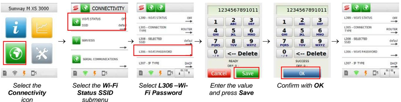
**Figure 43: Setting the network access password**
