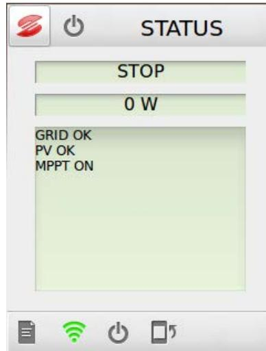
**Figure 60: Screen of the inverter Status menu**
